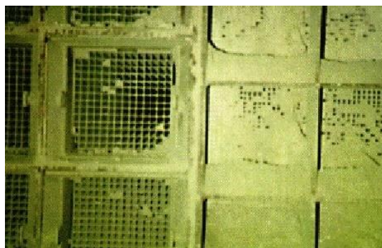
Dust Clogging and wear-out of catalyst
